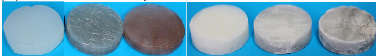
Fig. 1 - Image of samples for thermal conductivity measurement (from left to right): PW, PW+Al, PW+Cu, SA, SA+Al, SA+Cu
